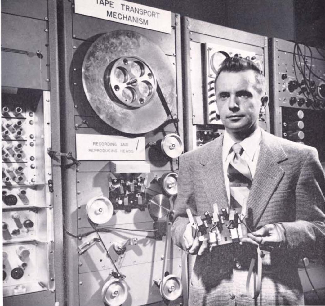
This recording "head" shown by Joseph Zenel, research engineer, is a vital part of RCA's magnetic tape recording apparatus used to record television programs both in black-and-white and in color
