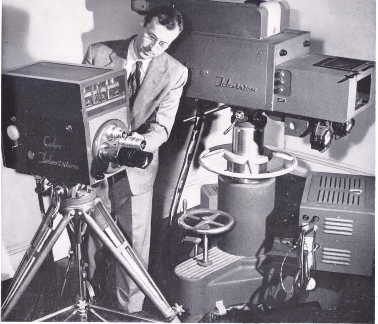
Under development by RCA engineers is this color camera which uses only one pickup tube
