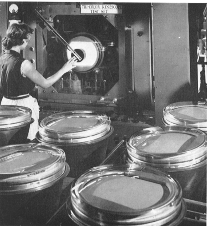
Tri-color television picture tubes in pilot production at the RCA plant in Lancaster, Pa., receive testing
